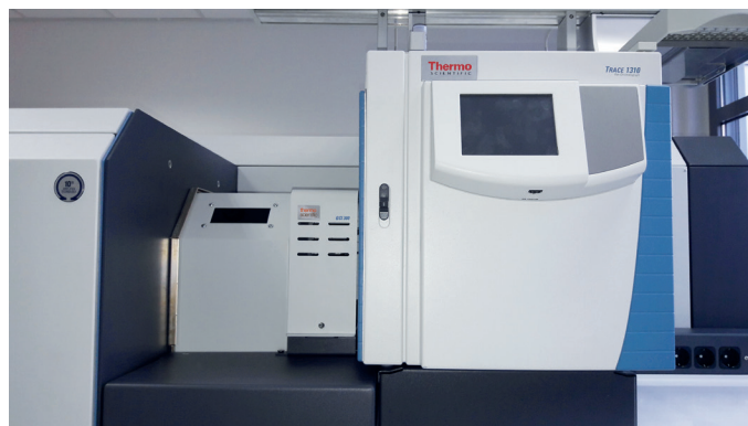
Figure 10. GCI 300 Interface between Trace 1310 GC and Neptune XT MC-ICP-MS.
