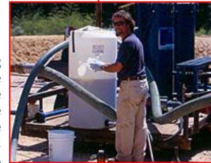
Preparing fluoresceine solution to be injected in the Frio Brine research project, Texas USA
