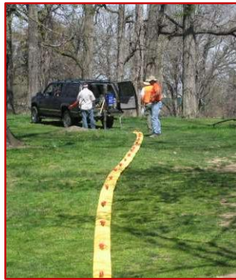
Near-surface seismic survey with geophones MASW technics photo: USGS
