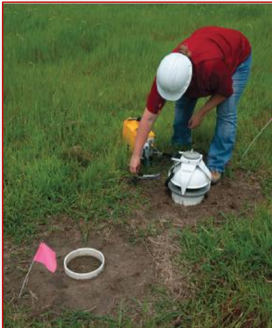
Measuring soil CO 2 fluxes with a chamber-based method
