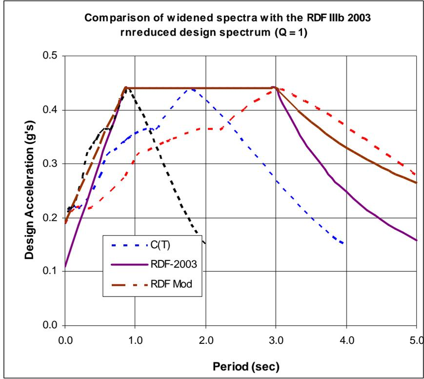
Fig. 6. Widened spectra  $C(T)$  (dashed lines) and design unreduced spectrum (solid lines)
