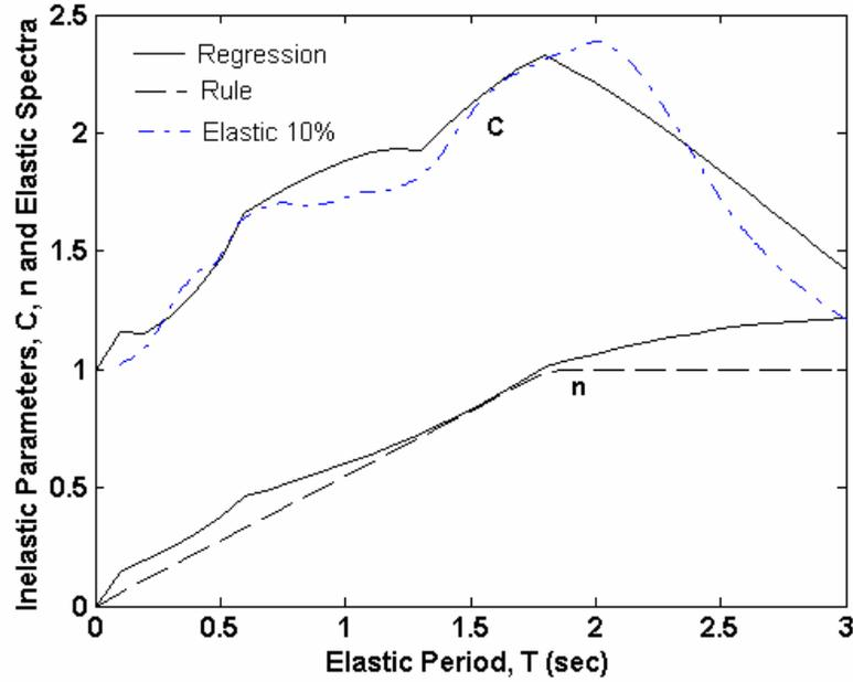
Fig. 4. Unreduced spectrum  $C(T)$  and power  $n(T)$  in Eqs. (2) and (3), determined with a regression fit
