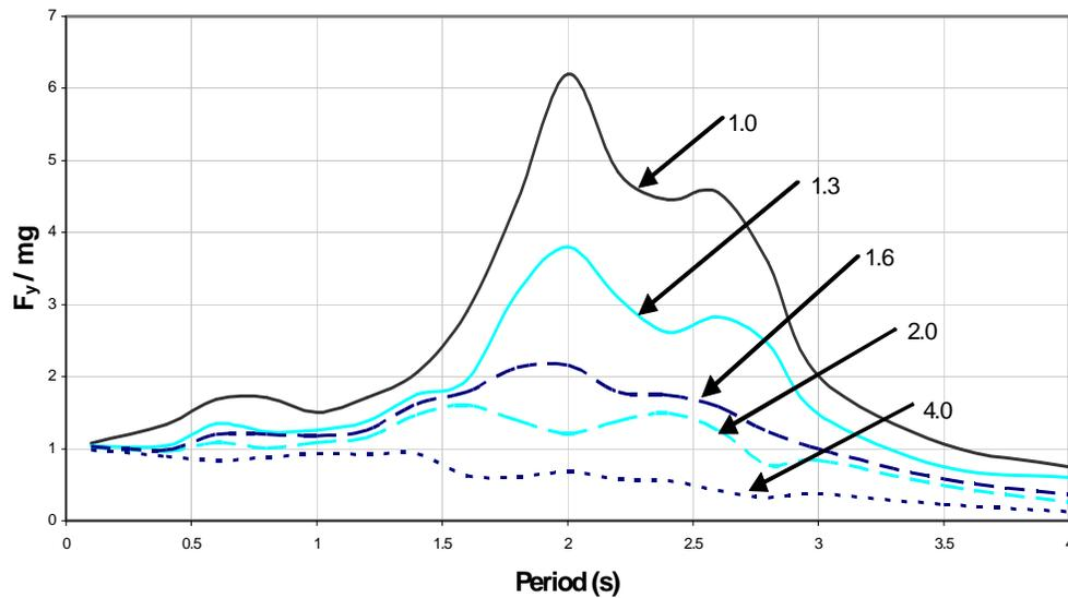
Figure 2. Inelastic spectra of the SCT 1985 record for different ductility ratios
