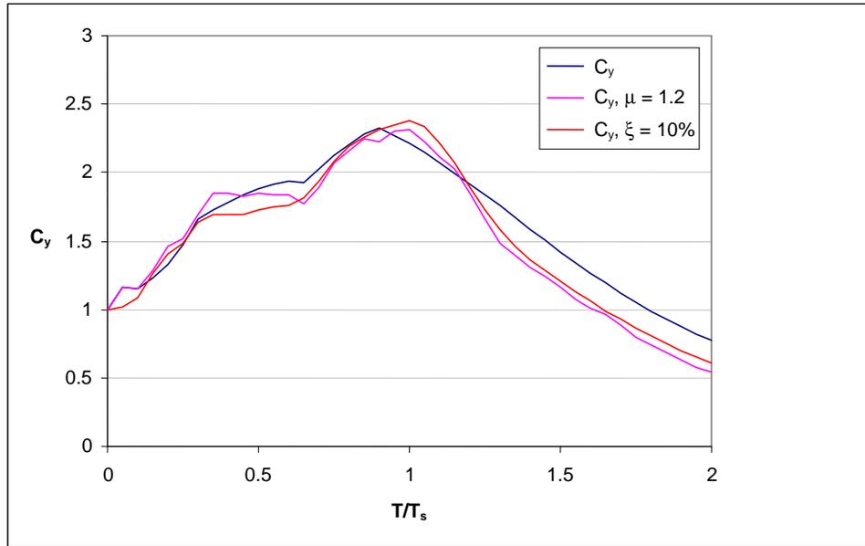
Fig. 5. Unreduced spectrum  $C(T)$  determined from a regression fit (solid lines), by 10 % elastic spectrum (dashed lines) and inelastic spectrum for  $\mu = 1.2$  (dashed-dotted lines).
