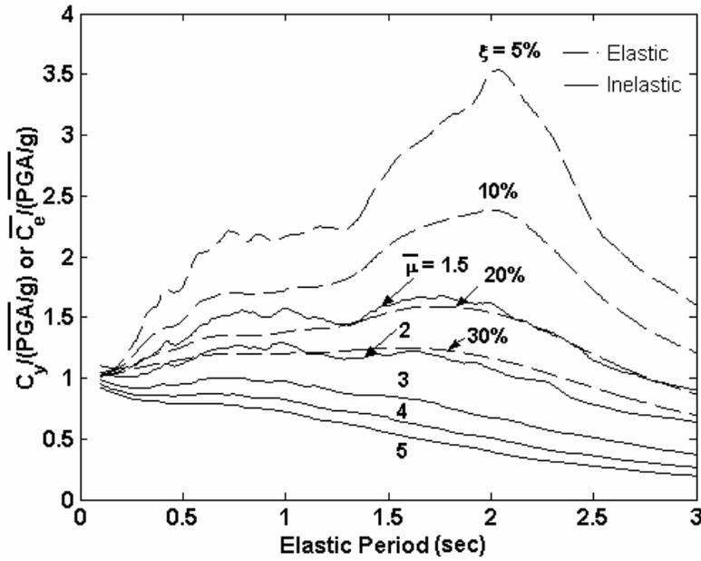
Fig. 3. Normalized spectra  $C_y(T, \bar{\mu})$  and  $\overline{C_e}(T, \xi)$  for different mean ductility ratios,  $\bar{\mu}$ , and critical damping ratios,  $\xi$
