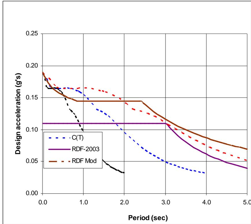
Fig. 9. Widened reduced spectra from Eq. 3 (dashed lines), RDF 2003 design spectrum (solid lines) and an example of a modified design spectrum (dash – solid lines), for  $Q = 4$
