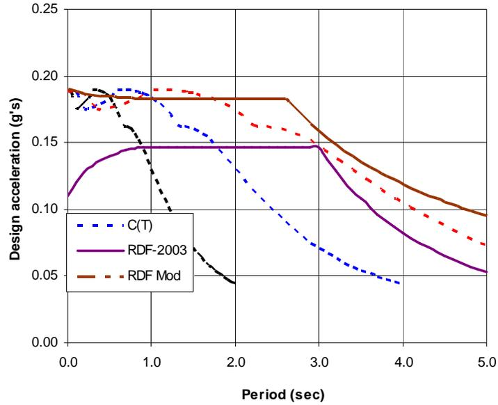
Fig. 7. Widened reduced spectra from Eq. 3 (dashed lines), RDF 2003 design spectrum (solid lines) and an example of a modified design spectrum (dash – solid lines) , for  $Q = 2$ .
