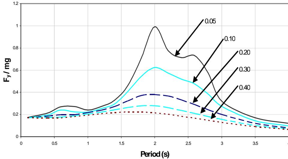
Figure 1. Elastic spectra of the SCT 1985 record for different damping ratios
