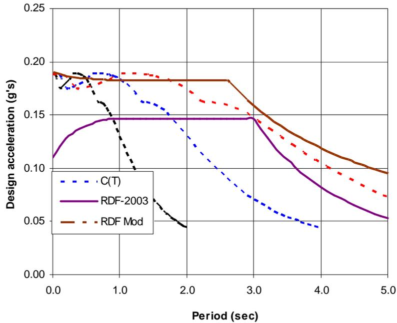
Fig. 8. Widened reduced spectra from Eq. 3 (dashed lines), RDF 2003 design spectrum (solid lines) and an example of a modified design spectrum (dash – solid lines), for  $Q = 3$
